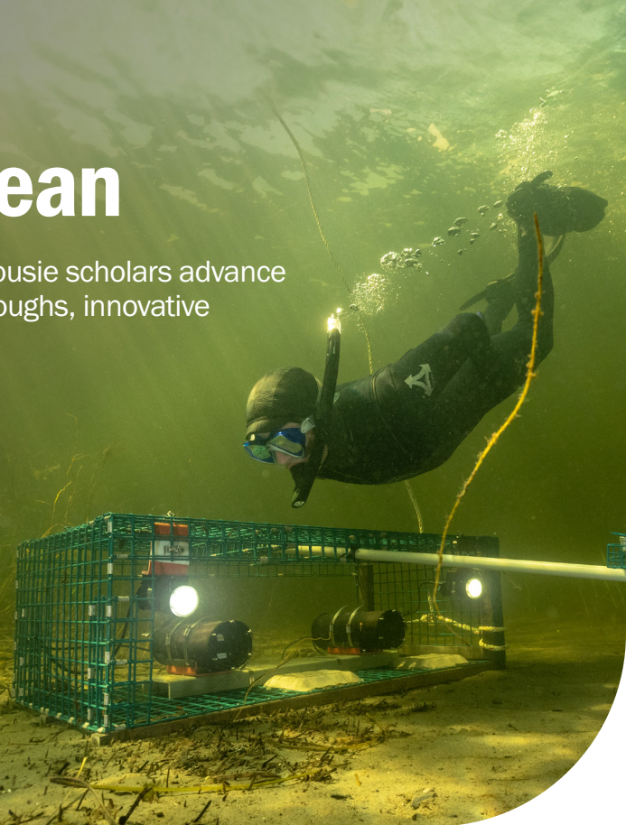
Remote underwater video camera on the edge of an eelgrass meadow. Photo Nicolas Winkler
